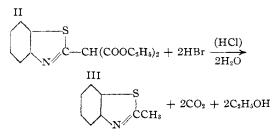
The product resulting from the loss of hydrogen bromide, and cyclization, forms a salt with alcoholic potassium hydroxide and also acts enolic toward a Grignard reagent. With hydrochloric acid, it undergoes hydrolysis and decarboxylation, to yield the well-known 1-methylbenzothiazole.
